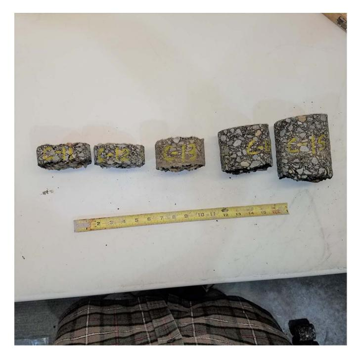
**Photo K:** Photo of asphalt cores C-11 to C-15 from left to right.
