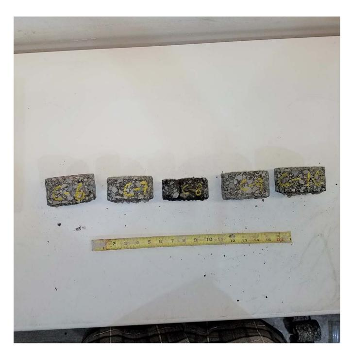
**Photo J:** Photo of asphalt cores C-6 to C-10 from left to right.
