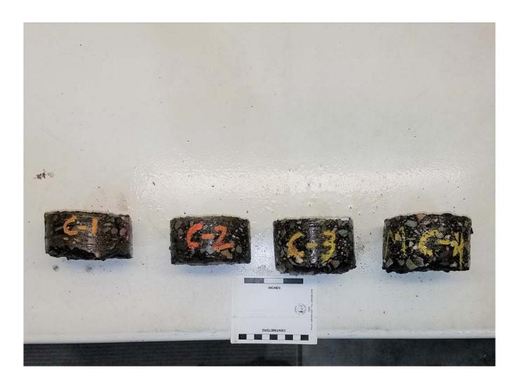
**Photo I:** Photo of asphalt cores C-1 to C-4 from left to right. Scale in inches and centimeters.
