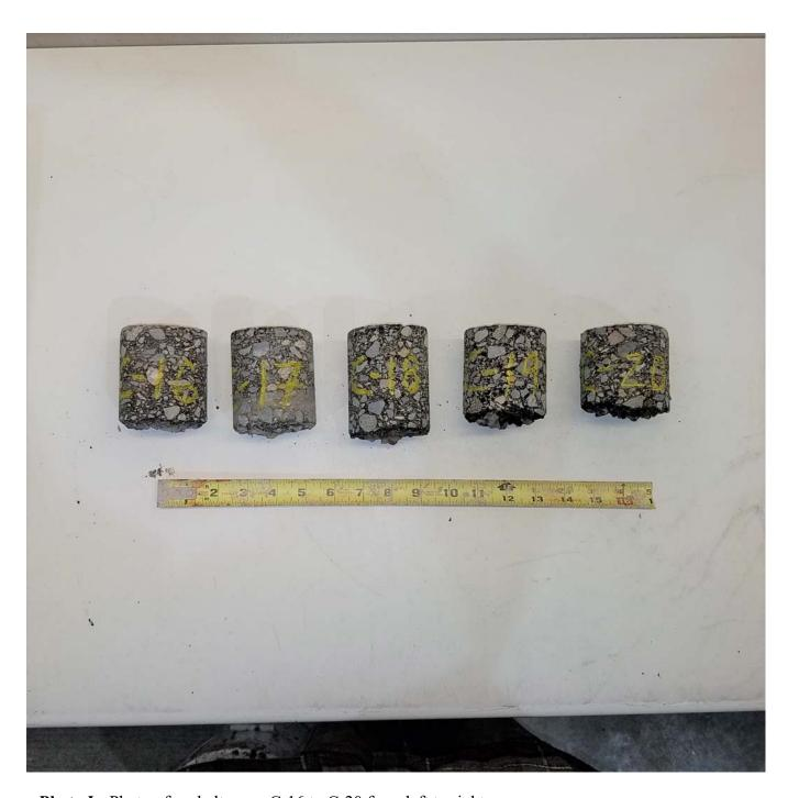
**Photo L:** Photo of asphalt cores C-16 to C-20 from left to right.
